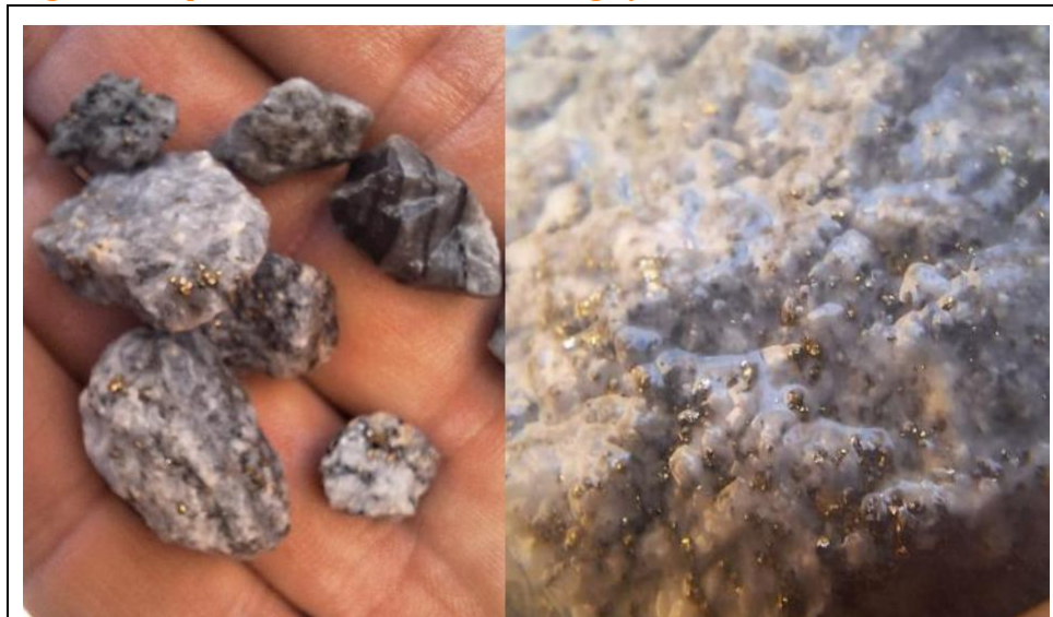
Figure 11: Sulphide metal mineralisation in the greywacke in the bedrock at Ibel South
