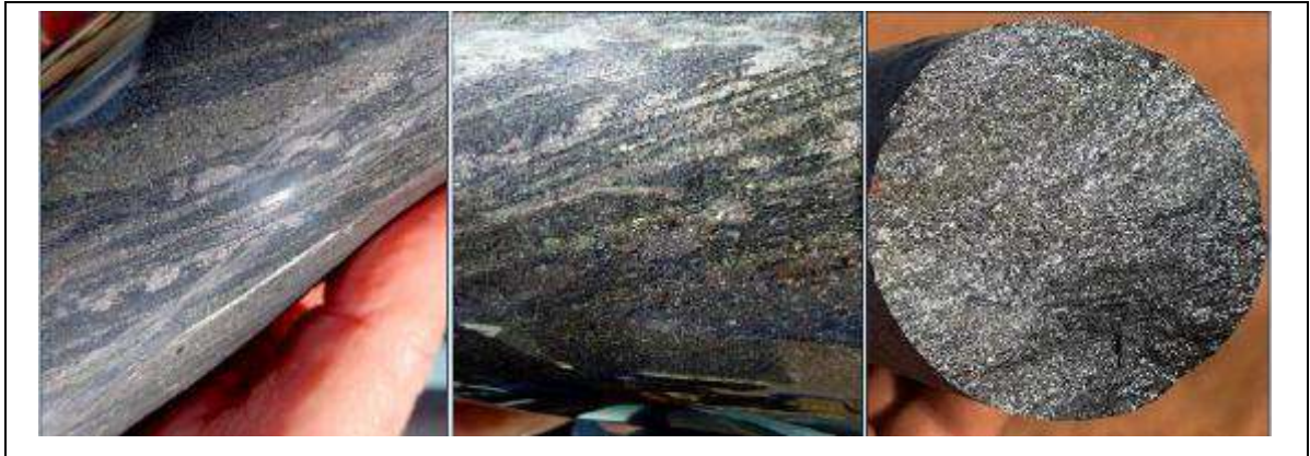
Figure 10: HQ drill core sample of coarse-grained recrystallised BIF containing 40%-45% magnetite content
