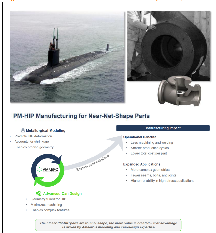
Figure 10: PM-HIP Provides an Alternative Route for Complex Components
